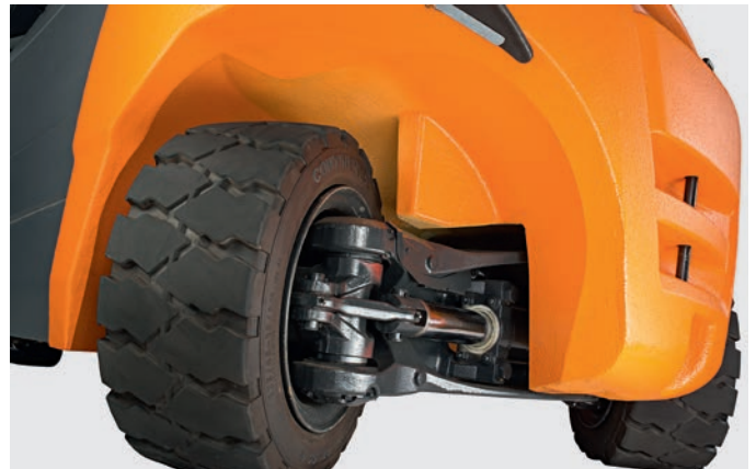
Manoeuvrable and stable high pendulum axle
