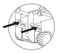
Position the forklift forks in position with the forklift pockets.
