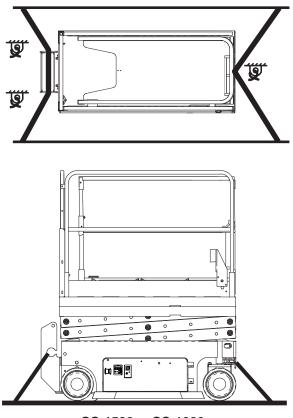
GS-1530 GS-1930 GS-1532 GS-1932 Inspect the entire machine for loose or unsecured items.
