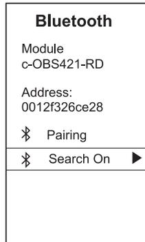
Exit the menu and check that the Bluetooth icon is no longer visible in the top left hand corner of the display.
