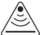
The overhead signal alert is triggered if vScan detects a significant signal radiating from above, for instance an overhead cable.
