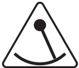
The swing alert will trigger if the angle of swing exceeds 30 degrees from the vertical. No alarm will be activated if the angle is more than 65 degrees from the vertical as it will be assumed that the locator is not in use at this time.
