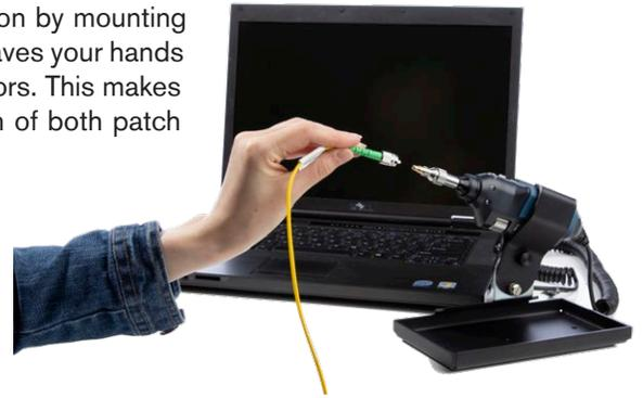
Inspecting and analyzing fiber connector endfaces has never been easier with this digital fiber inspection scope.
