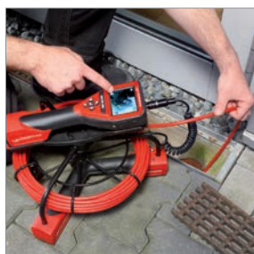
Inspection of rain drainpipes
