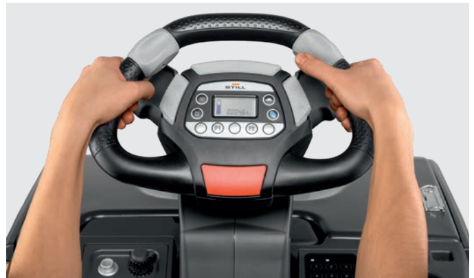
Thanks to the height-adjustable STILL Easy Drive steering wheel, all functions can be operated with ergonomic controls by right- and left-handed operators without changing grip
