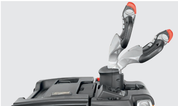
The flexibly adjustable working angle of 83° enables an ergonomic working posture of the tiller - and that for operators of any height
