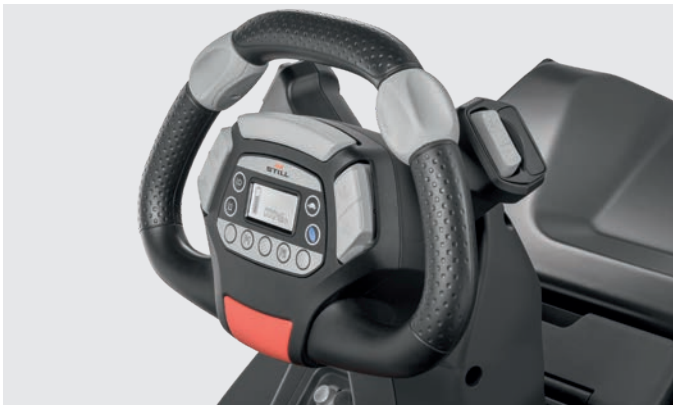
Simultaneous driving and lifting with the optional STILL Easy Move paddle shifters
