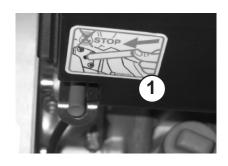
Turn the ignition key counter clockwise to the vertical position.
