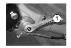
Control drive speed and direction of travel with the handle (1).
