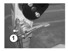
Press the switch off button (1) until the engine comes to a stop.
