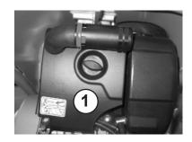
Remove the air filter insert (1) from the air filter enclosure Clean the air filter insert in accordance with the guidelines provided by the engine manufacturer, or replace if there is extreme fouling.
