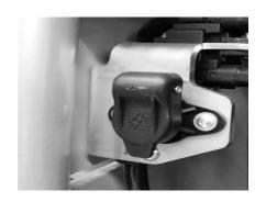
Insert plug into the charging socket.
