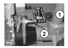
Fit the crane hook into the hinged lifting ring (1) and lift the machine onto the desired means of transport.
