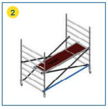
Mount the diagonal braces crosswise. Mount the work platform on one half of the 4th rung level (ensure that the trapdoor opens to the outside). Check the vertical and horizontal straightness using a level. If necessary, straighten using the adjustable legs.
