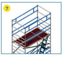
Install the bracing frames.
