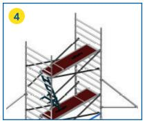
Mount the 7-rung end frame and lock it into place with the brace locks. Mount the diagonal braces to the end frame, with two on each side of the tower. Mount the ladder to the end frame and put the trapdoor platform into place (the trapdoor should be placed at the end of the tower opposite the trapdoor below).
