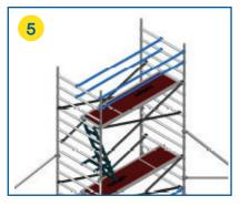
Use the horizontal braces as guardrails above the work platform.
