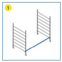
Install the castors and adjustable legs in the 7-rung end frame. Mount horizontal brace 1 to the end frame corner post as shown here (with the brace lock out).
