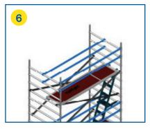
When the last end frame extension is in place, install the guardrail frame and lock it in place.
