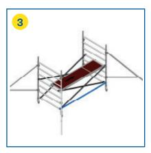
Fasten the stabilisers to all four corners of the tower.
