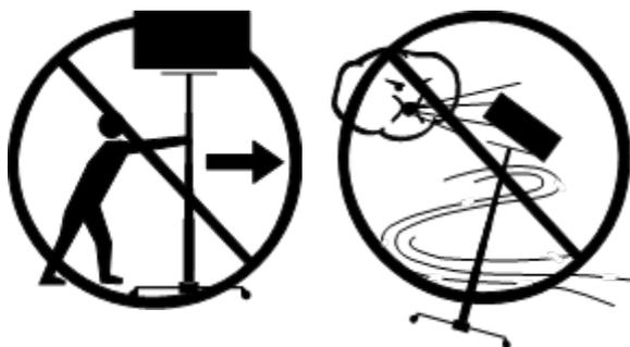
Do not operate the machine in strong or gusty winds. Increasing the load surface area will decrease machine stability in windy conditions.
