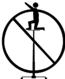
Do not raise the platform unless the machine is on a firm, level surface.
