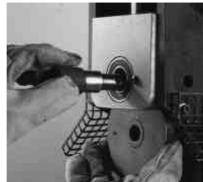
Fig 21: Pull out the upper shaft.
