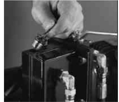
Fig 26: Filler plug oil reservoir.
