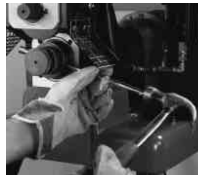
Fig 17: Remove locking pin.
