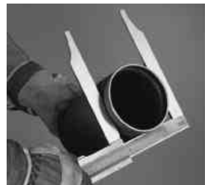
Fig 15: Measure the groove.
