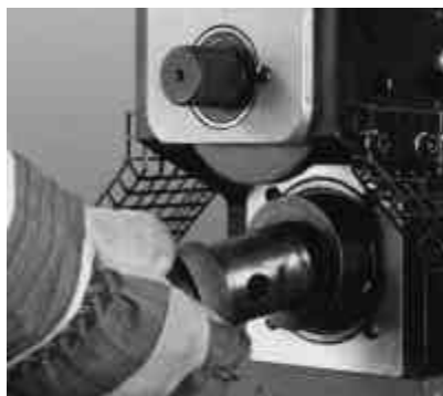
Fig 18: Remove lower roll.
