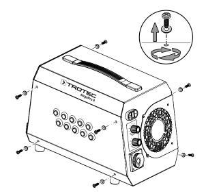
2. Remove the cover of the air filter.
