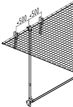
Image 52. Positioning of the Facade Attachment
