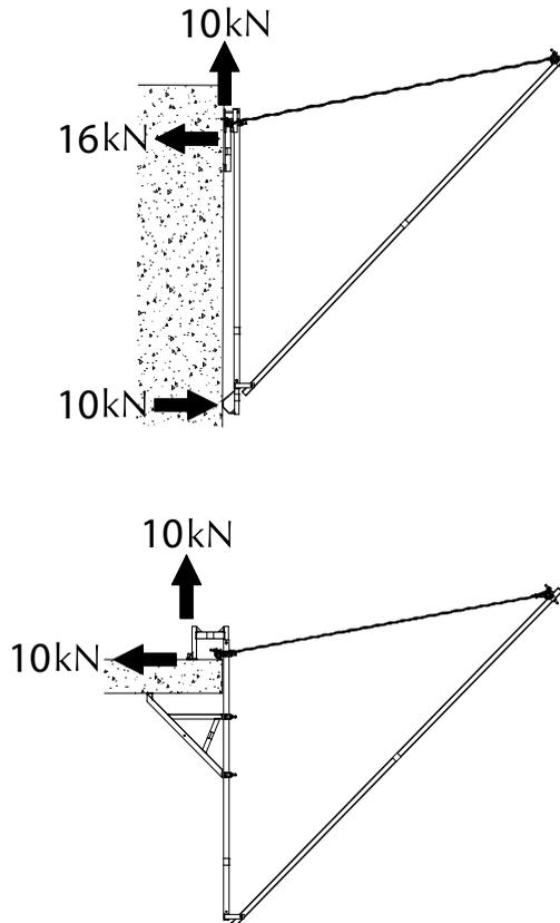
Image 42. Reaction forces, general, for wall/slab mounting
