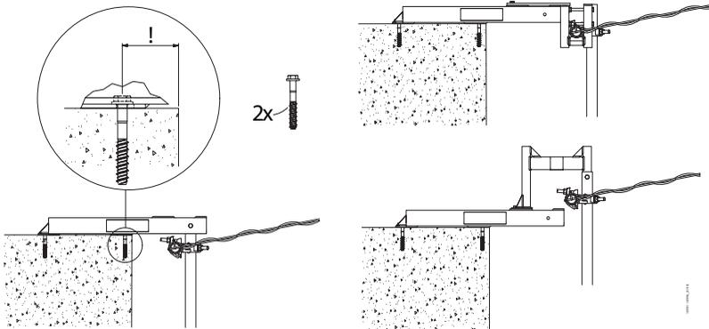
Image 19. Examples of assembly-Offset Beam
