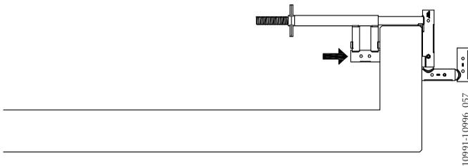
*Image 64. Attach a fastener in concrete upstand to secure Multi-Clamp*
