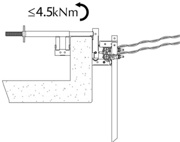
Image 44. Moment transferred to upstand using Multi Clamp
