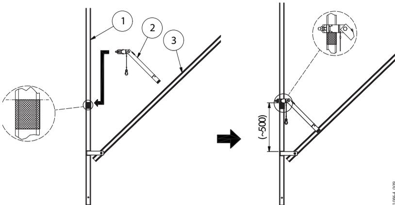
Image 9. Fitting the Wind Lock to the body
