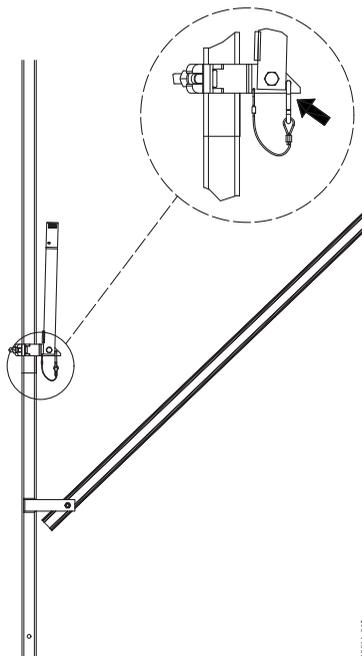
Image 15. Disengaging Wind Lock with Spring Hook
