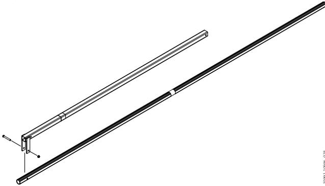
Image 28. Assembly of Frame and diagonal Tube
