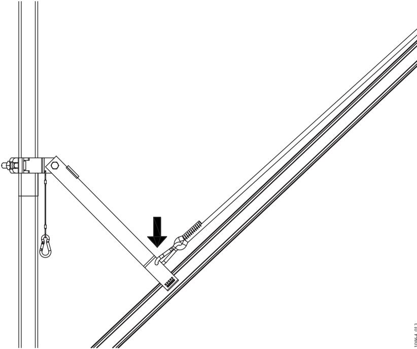
Image 13. Attached Maneuvering Rope on Wind Locks
