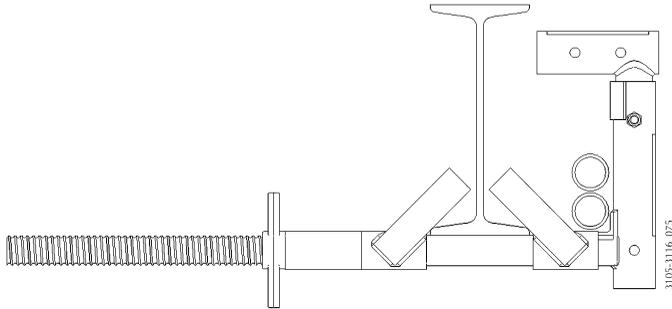
*Image 70. Overlap within the Steel Jaw Clamp with elbows*
