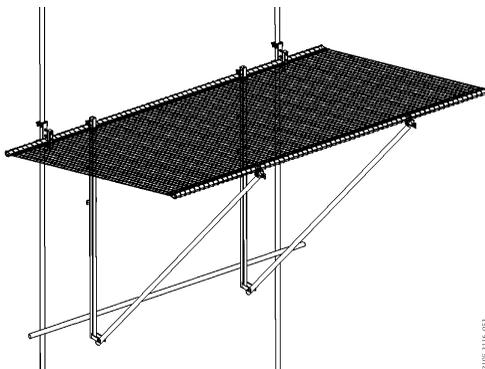
Image 58. Safety Net Fan installed on a scaffold
