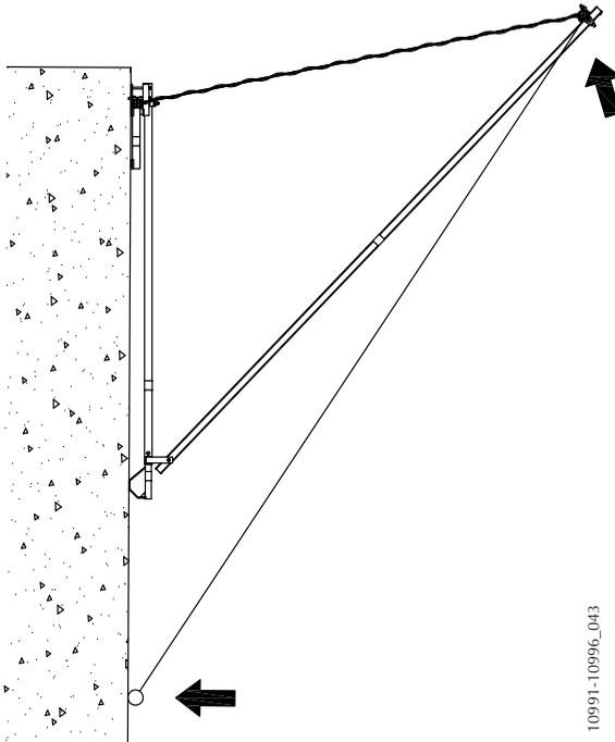
Image 46. Safety Net Fan tied to building with a rope
