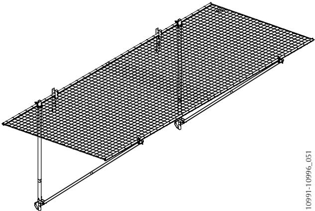
Image 54. The Safety Net Fan installed within the Facade Attachment
