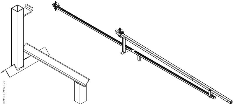
*Image 27. Positioning the Frames on the Assembly Aid*
