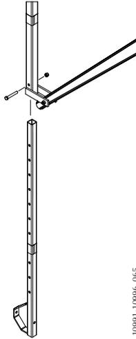
*Image 72. The Extension assembled in the Frame*
