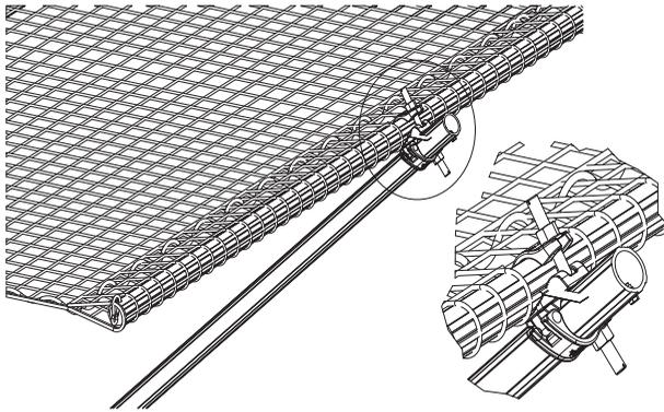
*Image 38. Assemble the outer Tube on the raking Tube*
