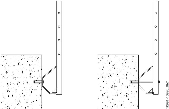
*Image 74. Variants of Extension anchored to slab*
