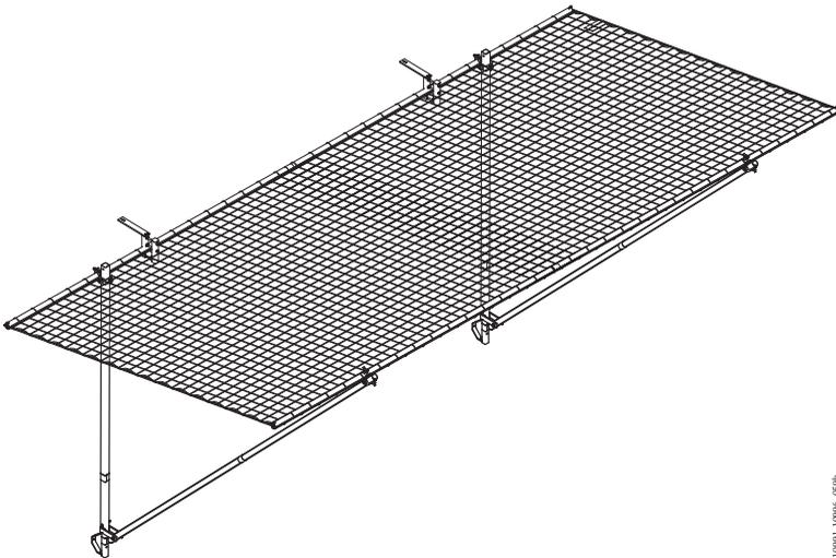
Image 62. The Safety Net Fan installed within the Loose Slab Attachment
