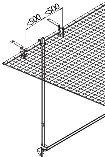
*Image 60. Positioning the Loose Slab Attachment*
