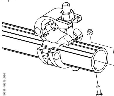
Image 30. The securing screw/nut
