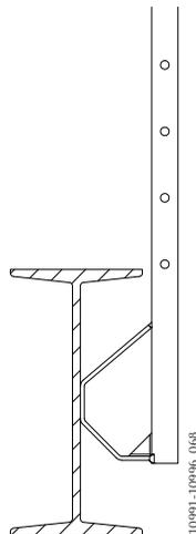
*Image 75. Extension supported on steel beam*
