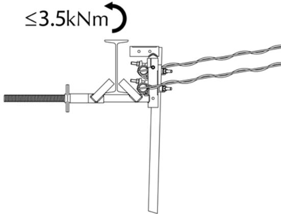
Image 43. Moment transferred to beam using Steel Jaw Clamp
