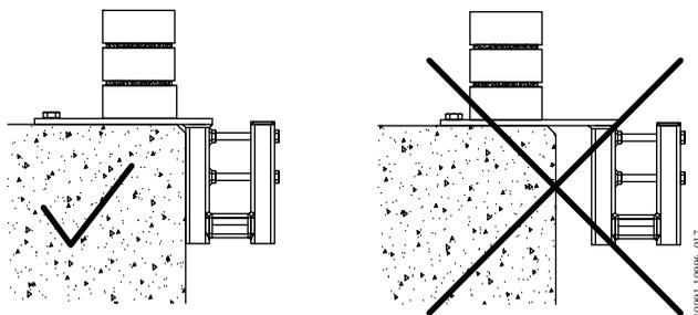
Image 17. Assembly of Loose Slab Attachment
