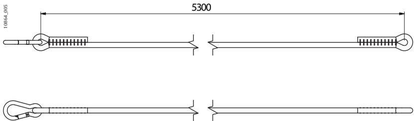
Image 5. Dimensions, Maneuvering Rope- Wind Lock
