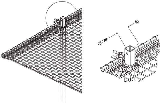
Image 37. The securing bolt/nut
