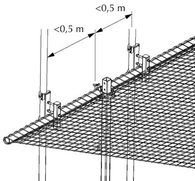
*Image 56. Positioning the Scaffold Attachment*
