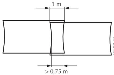
*Image 25. Fall-Arrest Safety Net Fan overlap*
