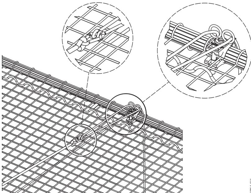
*Image 14. Fitting the Maneuvering Rope
