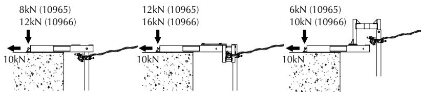
*Image 45. Reaction forces, Offset Beams*
