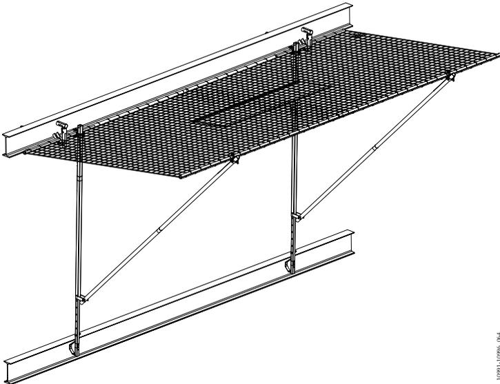
*Image 71. Safety Net Fan installed with Steel Jaw Clamps*
