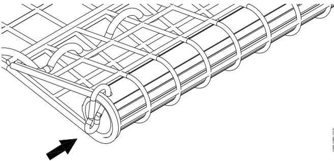
*Image 33. Secure the Net with snap hooks*
