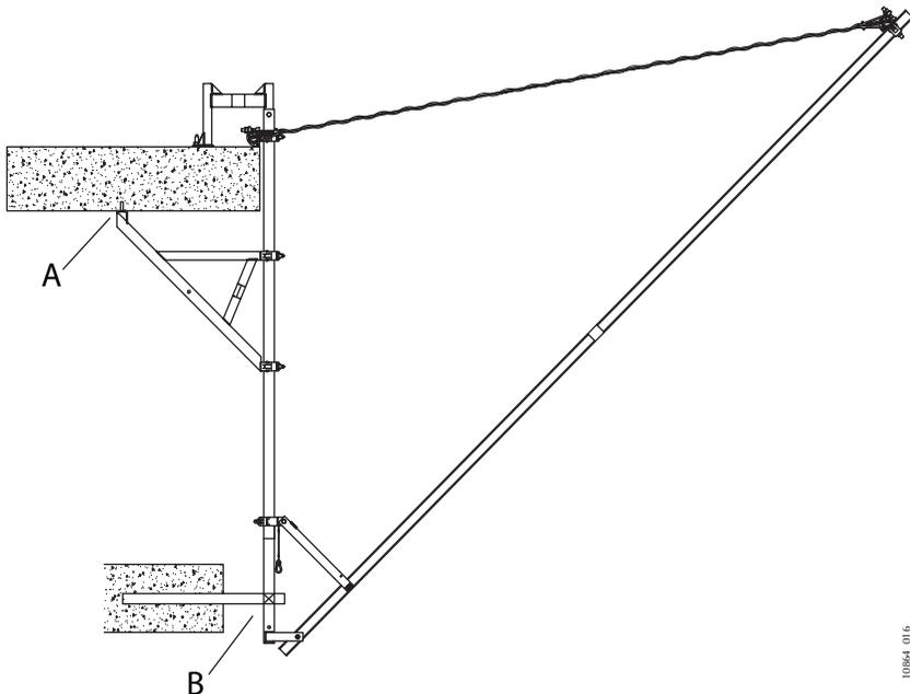
Image 16. Slab fitting option, anchor in A or B
