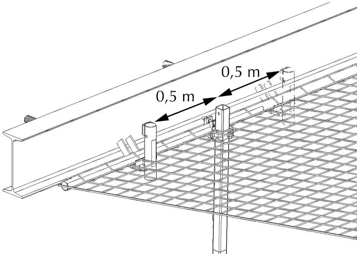
*Image 69. Positioning the Steel Jaw Clamps*
