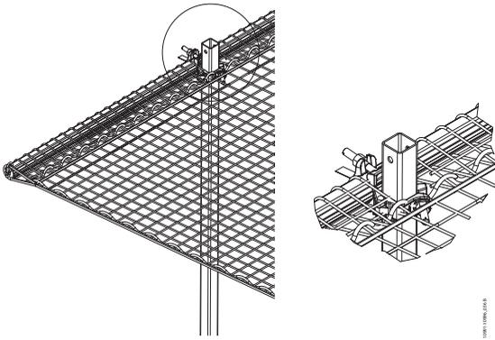
Image 36. Tube mounted in Frame coupler
