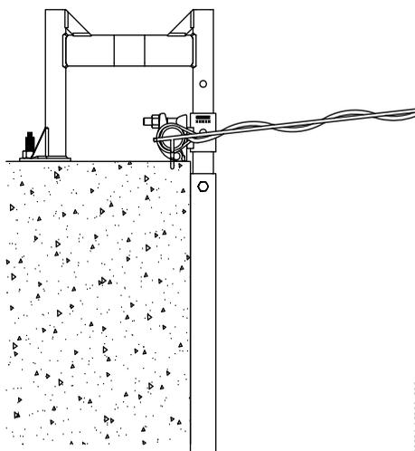
*Image 8. Normal assembly position of Adjustable Coupler on straight slab*
