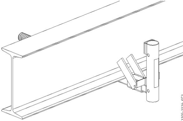
*Image 68. Steel Jaw Clamp on a beam*
