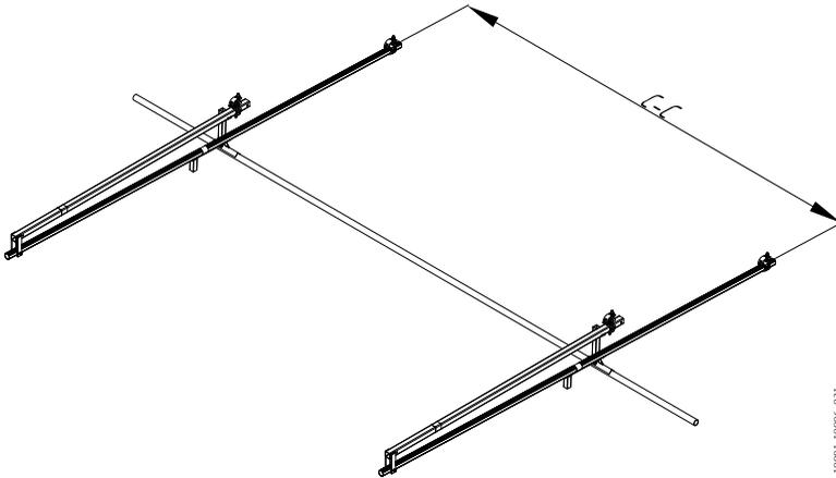
Image 31. Place the Frames with correct c-c spacing
