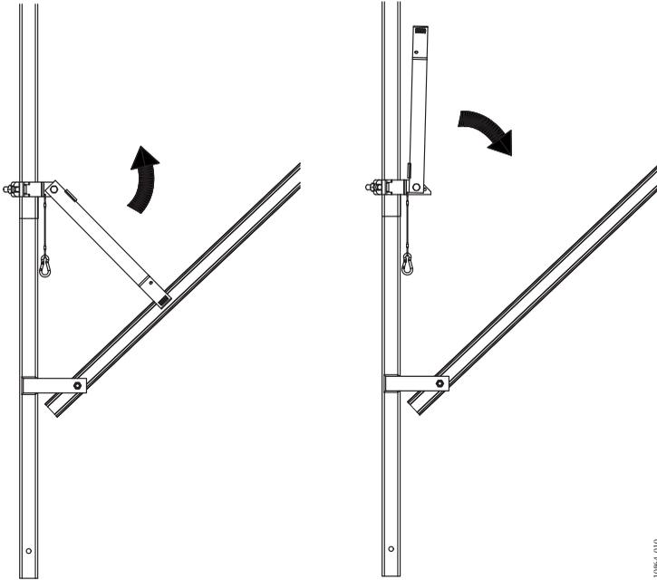
*Image 10. Activated and inactivated position*
