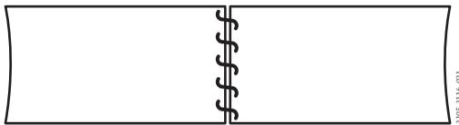
*Image 26. Joining Nets by lacing*
