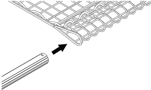
*Image 32. Inserting the outer Tubes into the Safety Fan Net*
