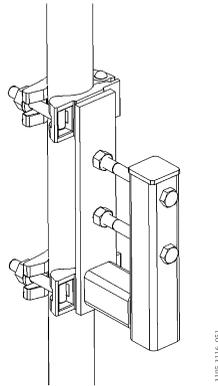
*Image 55. Scaffold Attachment installed on Tube*
