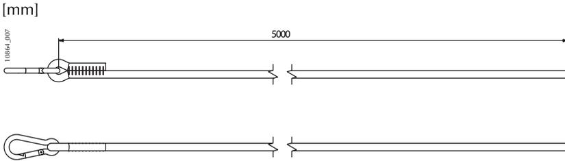
Image 7. Dimensions, Maneuvering Rope-Safety Net Fan
