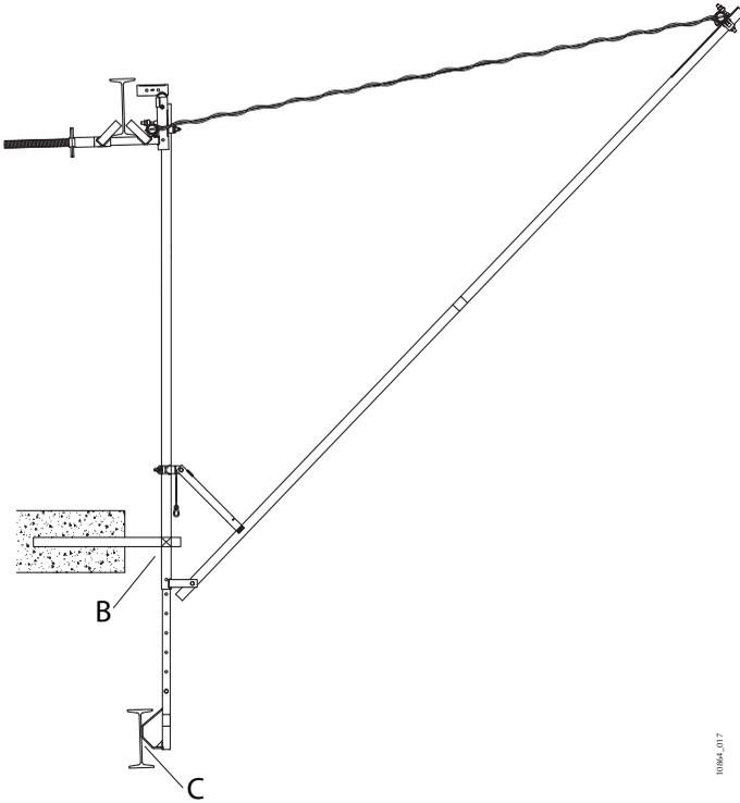
Image 17. Steel girder fitting option, anchor in B or C
