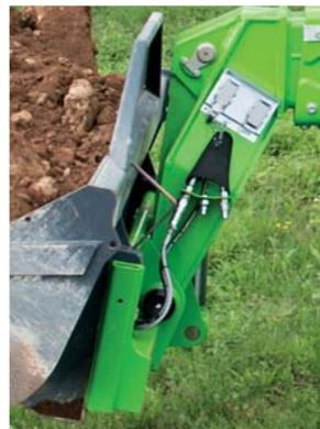
Pipes, electrical cables and auxiliary hydraulic are all located inside the boom for maximum protection.
