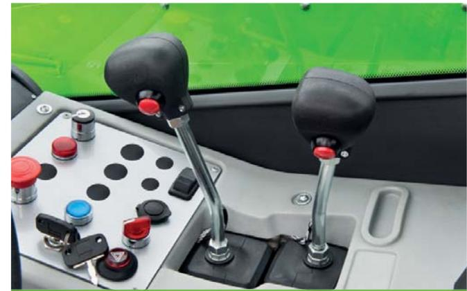
75 HP version: levers for operating the boom, carriage, attachments and boom side shifts
