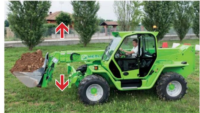
BSS hydro-pneumatic boom suspension (optional) engaged by the operator, it speeds up transfer, protects the load and improves productivity. It is deactivated at speeds <math>< 3 \text{ km/h}</math>.
