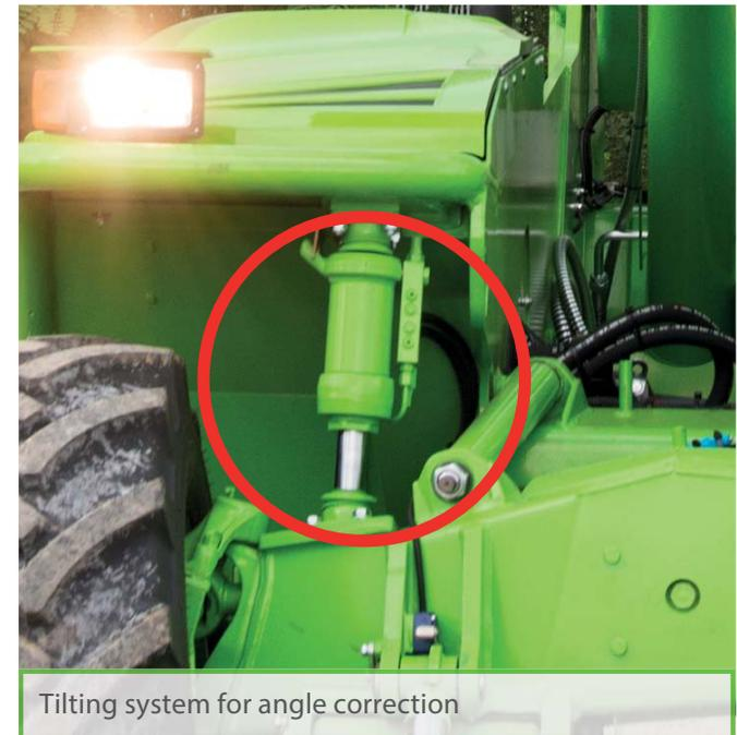
Tilting system for angle correction
