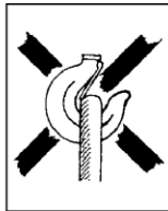
Fig 2 c Hook latch obstructed
