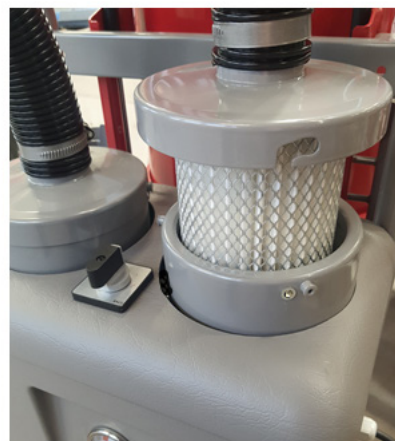
Figur 8 Carefully turn and lift the top cover HEPA filter Scan Dust 2900
