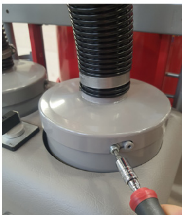
Figur 7 Top of the HEPA filter Scan Dust 2900 (2.), remove the two M5 bolt that secures the covers.
