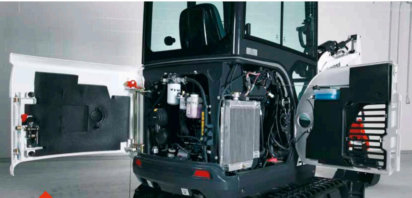
Side-by-side coolers for easy cleaning. Diagnostics are easy thanks to display error codes on control panel and service tool connection. With all openable covers the E17, E17z, E19 and E20z provide best-in-class access in their categories to all daily maintenance components and service points.
