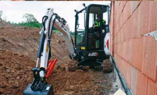
The Zero House Swing (ZHS) concept enhances Zero Tail Swing (ZTS) functionality by further protecting the front upper structure corners turning within the swing circle. ZHS functionality provides 320° of free rotation while working close to any object.
