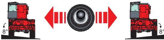
**+/-8°** level correction on the front axle
