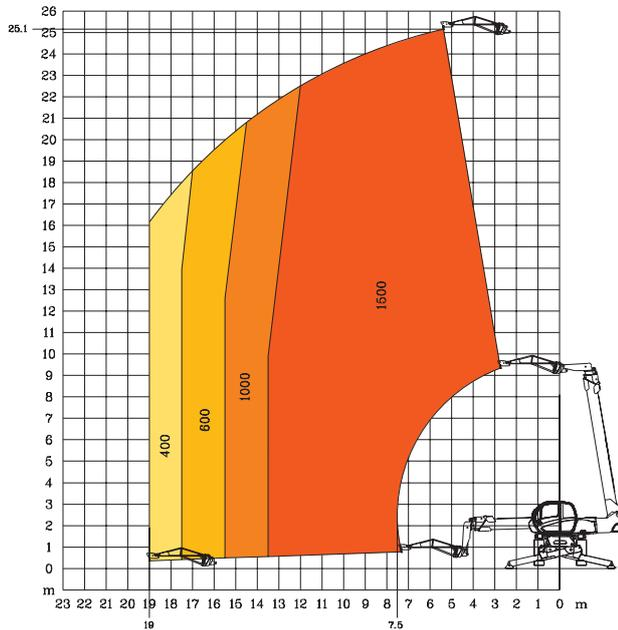
Rotation on extended stabilizers with **365/1000 kg platform**
