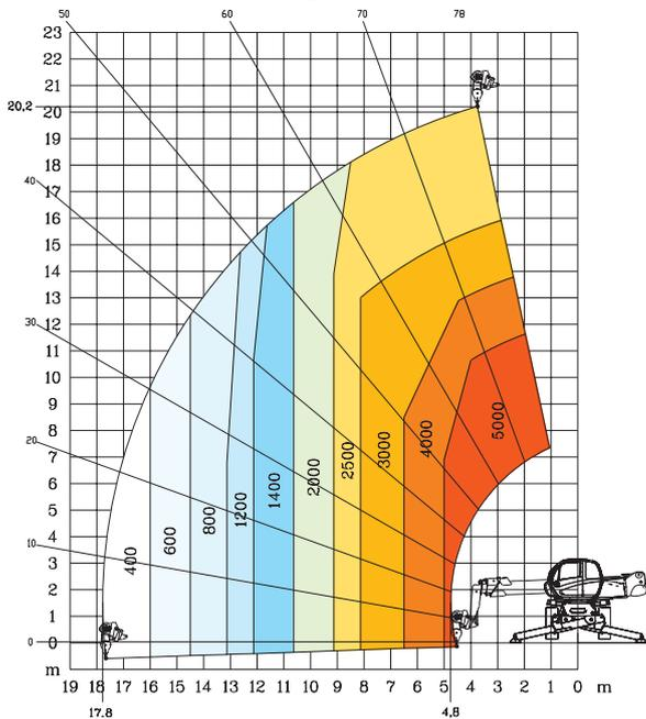
Rotation on extended stabilizers with **1500 kg jib**
