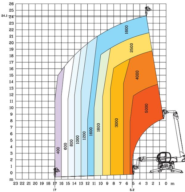
Rotation on extended stabilizers with **1500 kg jib**
