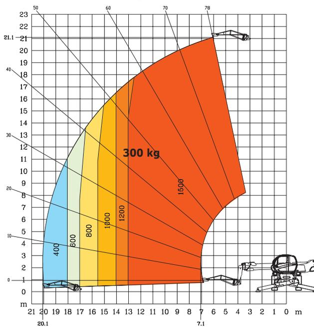
Rotation on extended stabilizers with **365/1000 kg platform**
