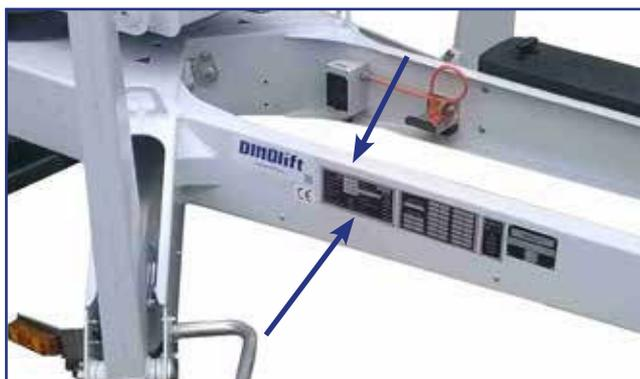
The nameplate of the trailer is located on the tow-bar, on the right-hand side of the nameplate of the lift, as shown in the picture.
