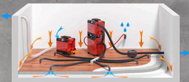
A turbine that suction dries a floor construction with water separator and combi filter.
