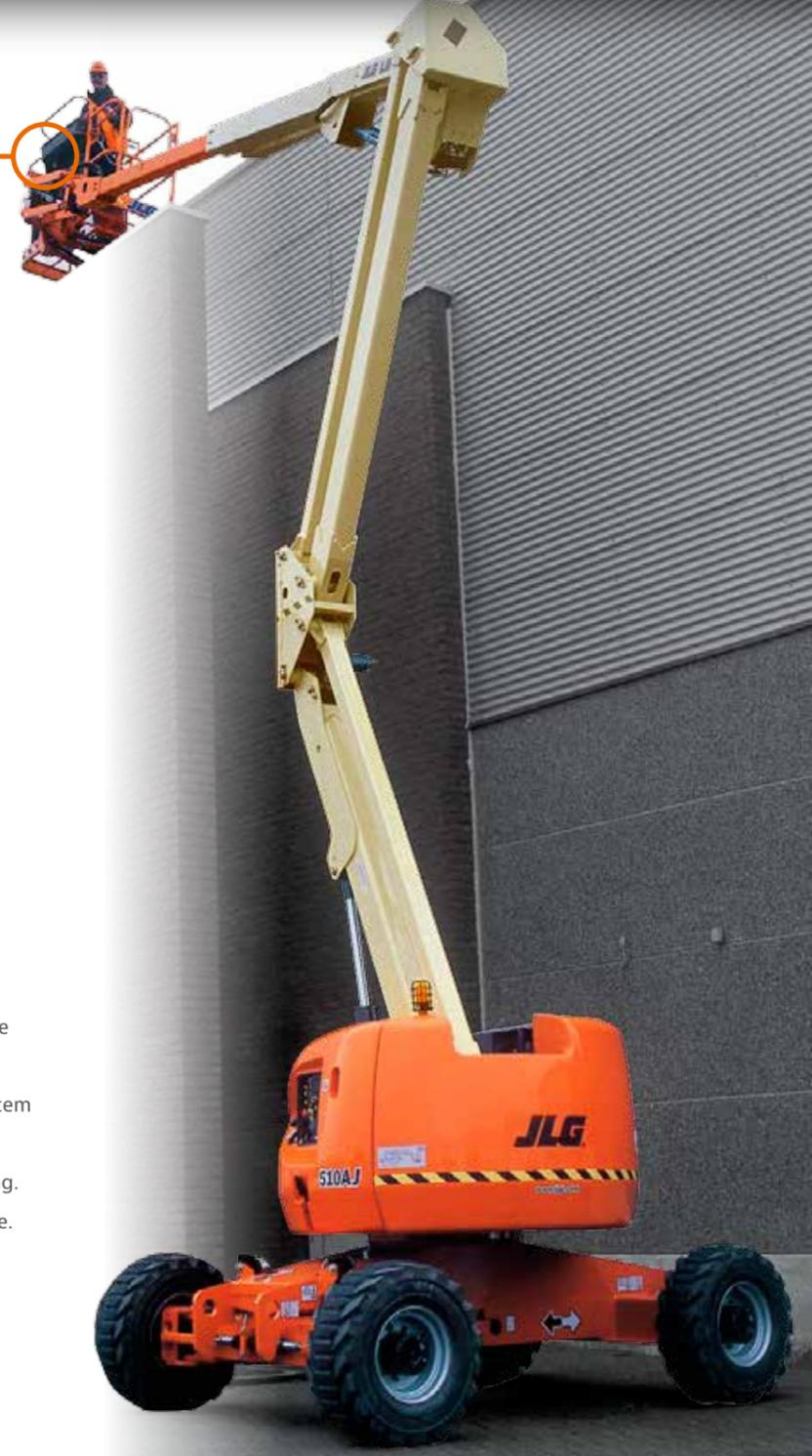
With up to 18 m of working height and an outreach of 9.48 m, the 510AJ boosts your productivity while getting you in those hard-to-reach areas. Standard four-wheel drive and oscillating axle provide superior terrainability. A work envelope with an articulating jib and 7.67 m of up-and-over height makes tricky corners no problem. The patented JLG® Control ADE® (Advanced Design Electronics) system, helps improve performance.
