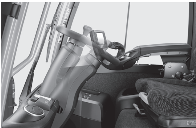
Individual adjustment of the steering column
