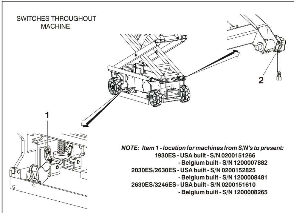
1. Pothole Switch (Typical on opposite side of machine)
