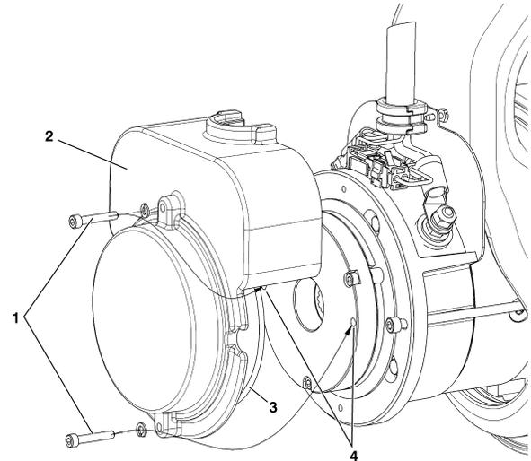
**Figure 4-5. Manual Disengage**
