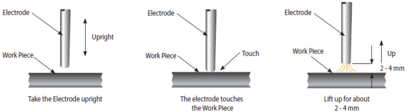
**Scratch technique** - Drag the electrode and scratch the work piece as if striking a match. Scratching the electrode may cause the arc to burn along the scratch path, so care should be taken to scratch in the weld zone. When the arc is struck adopt the correct welding position.
