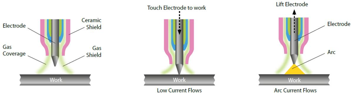
The Jasic Arc range allows the tungsten to be in direct contact with the work piece with minimal current so as not to leave tungsten deposits. Once contact has been made the tungsten can then be lifted away 2-4mm from the work piece and the welding arc is then established.
