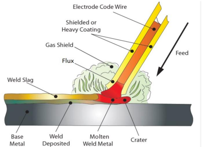
When the electrode is moved along the work piece at the correct speed the metal core deposits a uniformed layer called the weld bead.
