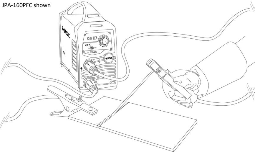
After connecting the welding leads as detailed you will need to switch the power switch on the back panel to "ON".
