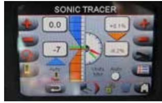
Sonic Tracer: To be installed on 244 cm and 274 cm Graders with ACD. Loader must be equipped with the Deluxe panel.
