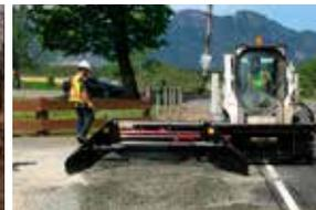
Soil and Asphalt Spreader
