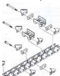
**\*IMPORTANT: WHEN INSTALLING SPACER KITS, A TRENCH CLEANER ADAPTER MUST ALSO BE INSTALLED.**
