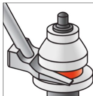
Use Bobcat **6678073**, **6678074** tools for extracting worn bits from attachment when they need to be replaced.
