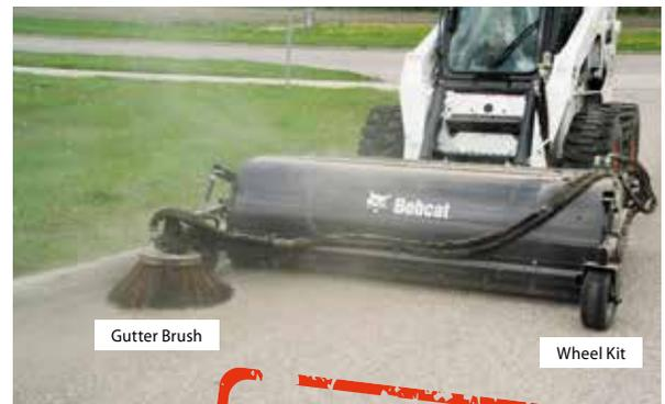
WHEN GOING FORWARD OR IN REVERSE WITH THE MACHINE, FOR BEST RESULTS, BRISTLES MUST SPIN COUNTER CLOCKWISE. PREVENT ANY DUST WITH THE OPTIONAL WATER KIT.
