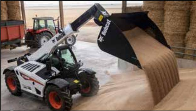
**Description:** The large volume of Bobcat Light Material Buckets is designed for loading and handling a variety of light materials such as mulch, snow and grain.
