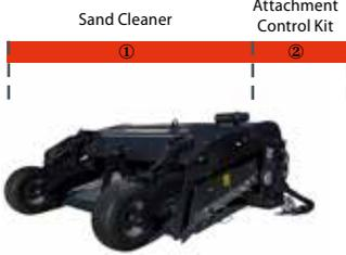
Sand Cleaner: Comes standard with a 15x15 mm grid. Loader must be equipped with an Attachment Control Kit.
