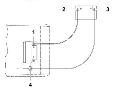
The following connection sequence must be used when starting with an external battery:
