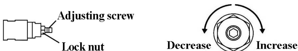
Fig. 6-5 Adjustment of relief valve
