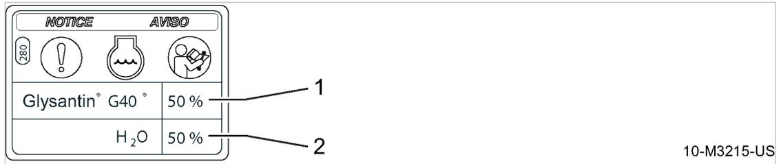
Fig. 40 Recommended mixture ratio for coolant
