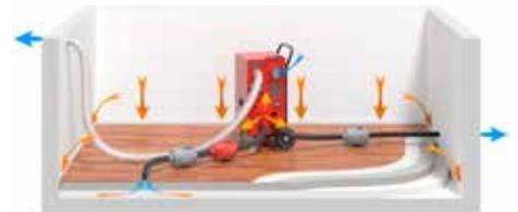
**Suction drying** should always be used as a first stage when drying floors on concrete slabs, where the water has leaked down into the fill or insulation under the floating floor. (The image shows CTR K150XT)
