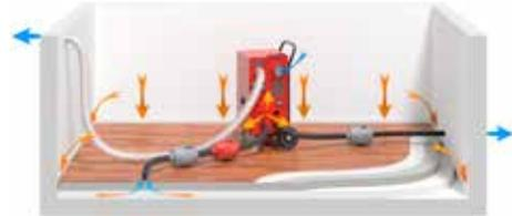
**Suction drying** should always be used as a first stage when drying floors on concrete slabs, where the water has leaked down into the fill or insulation under the floating floor.
