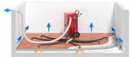
**Pressure drying** is one of the most effective and fastest commercially available methods for drying layered structures. (The image shows CTR K150XT)
