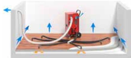
**Pressure drying** is one of the most effective and fastest commercially available methods for drying layered structures.
