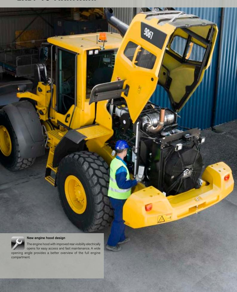
Time means money on site. That's why the new, electrically opening, engine hood is even easier to access for fast maintenance and service checks. Volvo's high-tech MATRIS and VCADS Pro software offers more in-depth engine and machine operation analysis to increase your uptime.
