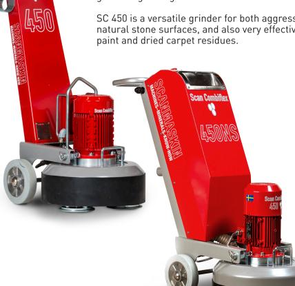
Both SC 450 and SC 450NS is a flexible and easy to use grinding machines, perfect for the rental market and smaller sized jobs with space constraints. These grinders are light, yet durable, being constructed almost 100% from steel. The spring-steel flex heads reduces vibrations, and allows the machine to grind rough surfaces with minimal effort for the operator.
