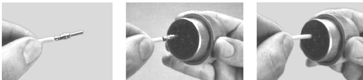
Figure 7-14. HD/HDP Contact Installation
