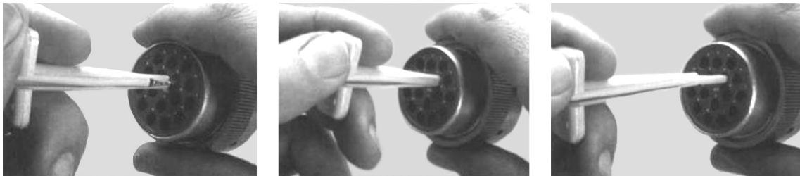
Figure 7-16. HD/HDP Contact Removal
