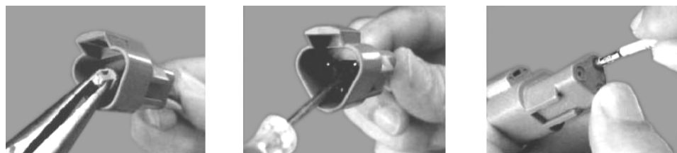
Figure 7-13. DT/DTP Contact Removal
