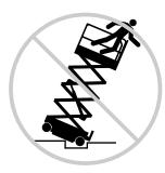
Do not drive the machine on or near uneven terrain, unstable surfaces or other hazardous conditions with the platform raised.
