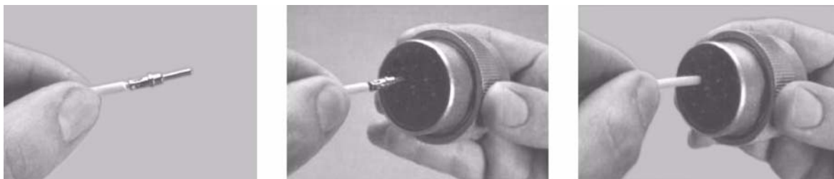
Figure 6-14. HD/HDP Contact Installation
