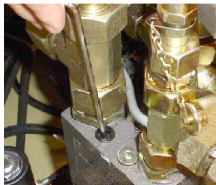
Figure 4-30. Proportional Valve Pressure Adjustment
