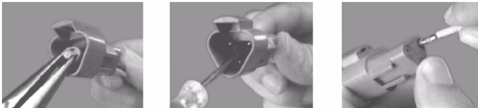
Figure 6-13. DT/DTP Contact Removal
