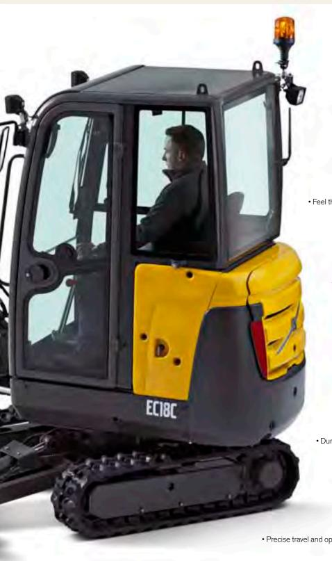
Operate in a protected TOPS/ROPS/OPG1 safety structure.
