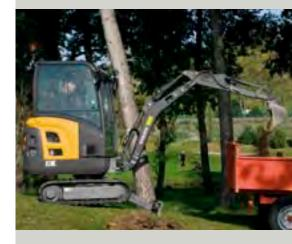
Protected, smartly-positioned boom cylinder.
