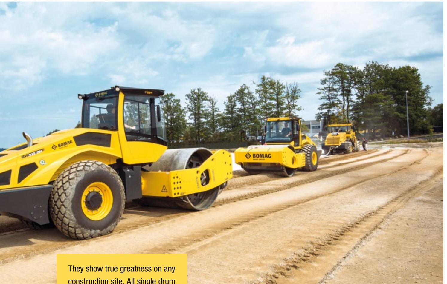
They show true greatness on any construction site. All single drum rollers in the heavyweight class have a working width of 2.13 metres. Depending on the equipment, the BW 226 is particularly impressive with its special depth effect or even rock-crushing capabilities.
