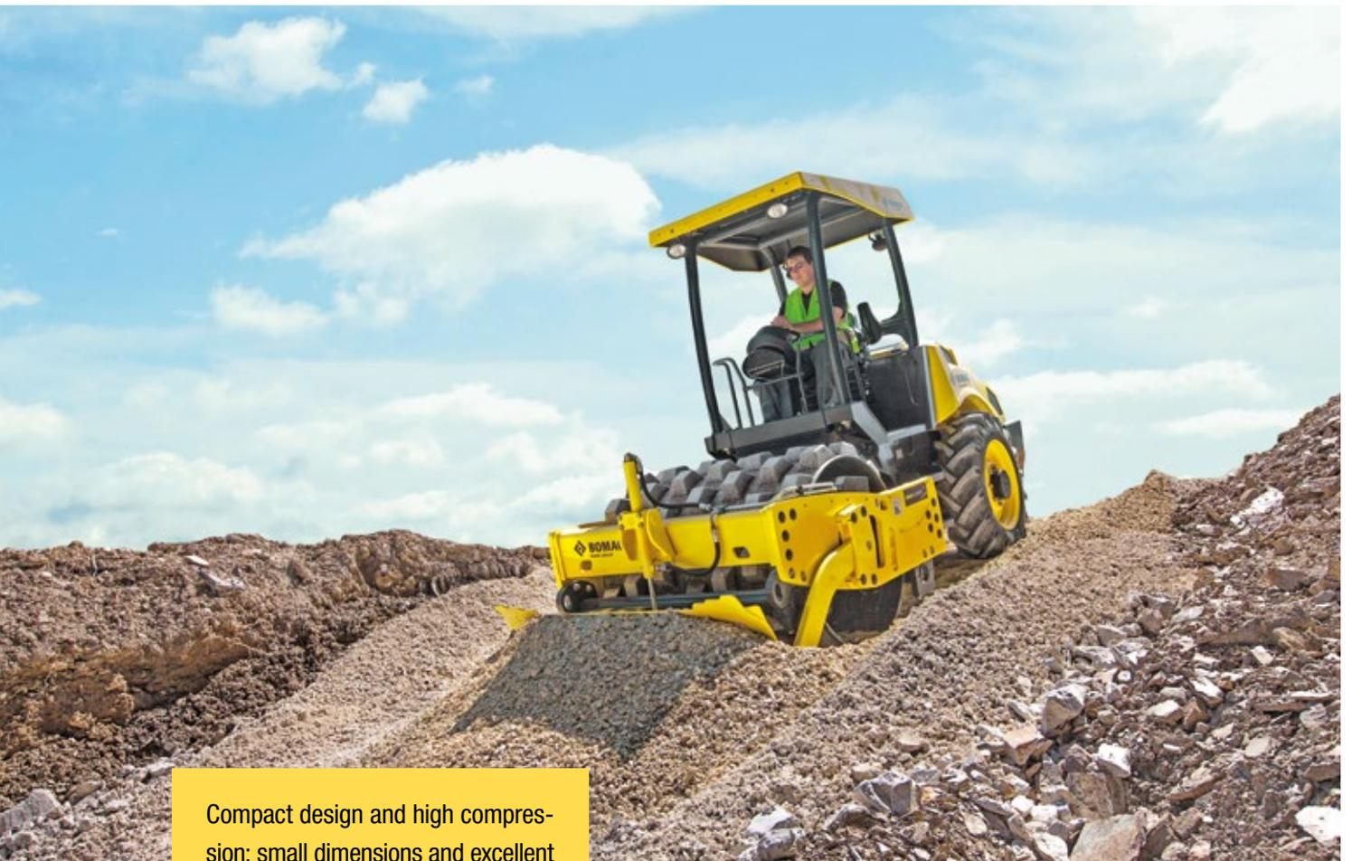
Compact design and high compression: small dimensions and excellent manoeuvrability combined with a high compaction performance make the single drum rollers the perfect choice for inner-city sites.
