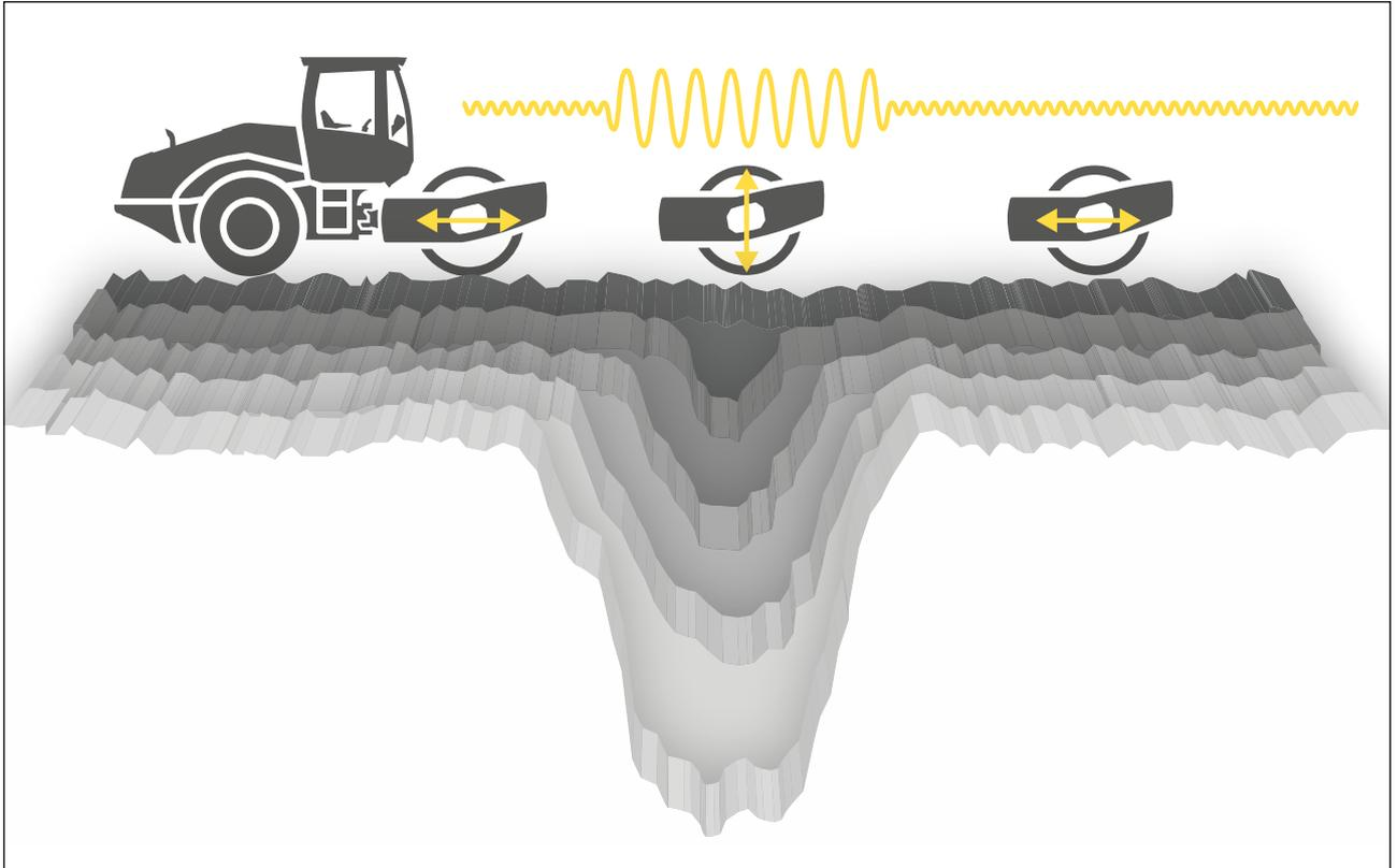
VARIOCONTROL automatically adjusts the amplitude to the degree of compaction.
