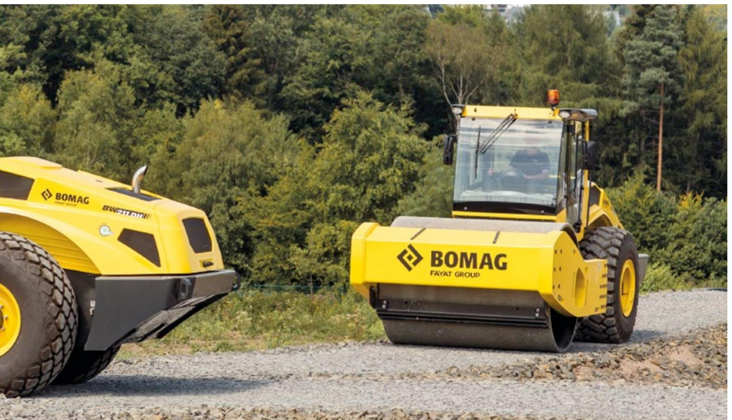
Reliability under the toughest conditions: with the manual slip control in the D machines and the double pump drive in the DH/PDH machines, Bomag sets new standards in the gradeability of single drum rollers.
