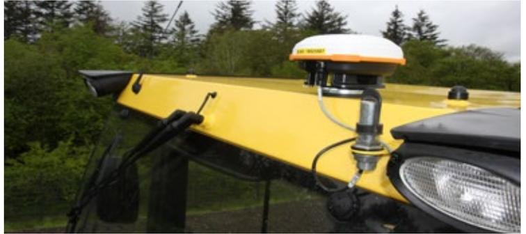
Increasing precision: the BOMAG GPS antenna.
