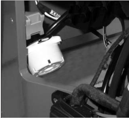
Fig. 153: Backup warning system
