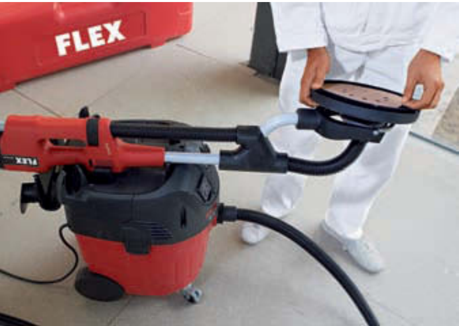
Simply place the Giraffe® on the rest and then you can conveniently change the abrasive or sanding head.
