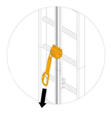
A simple down tension automatically locks the runner in its position
