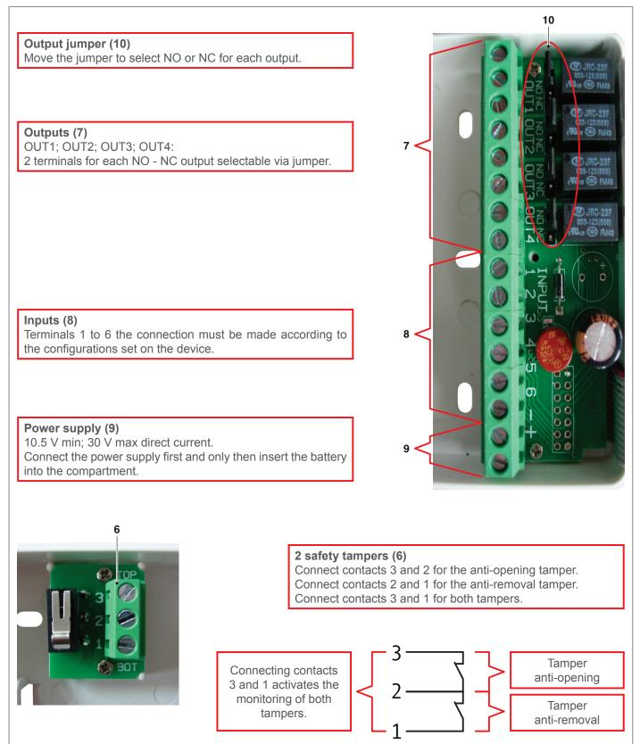
The **GSM-00** can be powered by the internal buffer battery alone for the time needed for configuration.
