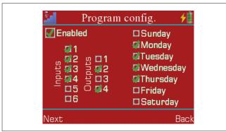
On the next screen, you can set the time and the inputs and outputs to be enabled/disabled by ticking the relevant boxes.
