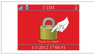
To unlock the dialler, tap the padlock in the centre of the screen and enter the administrator password (default setting "12345") using the touch keypad. Then tap confirm in the bottom right corner.
