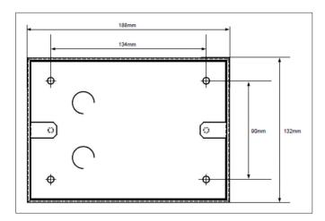
The back of the controller has a series of 20 mm holes at the top, rear and bottom.
