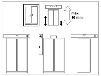
If necessary, level the product by adjusting the support feet.
