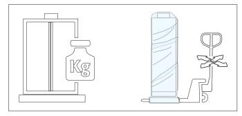
Use a pallet truck to move the product, which must be placed vertically and be secured and protected against slipping up to its final installation site.
