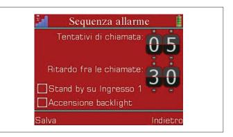
If "Standby on input 1" is ticked, input 1 works as a total dialler block, so it will not react to any alarm while this input is in alarm state. In these conditions, "Standby" appears on the main display to signal the dialler is not active. In the status SMS ("status" command), the text "StBy enabled" was added to the "System:" row if the function was enabled from the menu. The system status (standby or otherwise) is therefore visible on the "Inputs" row.
