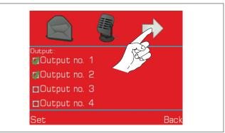
The **alarm sequence** of each trigger follows the order in which actions are entered. If more than one call actions occurs, the **GSM-00** will attempt to call all associated contacts. In case of a failed or unanswered call, after finishing the other calls it will make 5 more attempts as per the default setting (editable in "Set the alarm call sequence" a pag. 35 Justrite®) to call back the numbers that did not answer.
