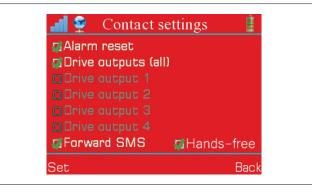
The contact settings are for assigning special remote control privileges to some contacts or forwarding messages the **GSM-00** receives to the corresponding number:
