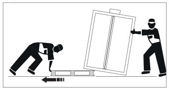
After removing the pallet, lower the cabinet slowly and smoothly to avoid damaging it.
