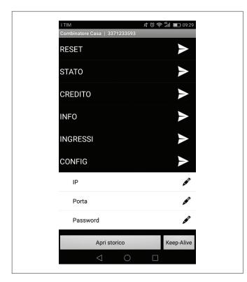
The "Keep-Alive" button at the bottom right of the screen allows you to set up a monitoring system based on "STA-TUS" messages. The dropdown menu is for selecting the operating mode.
