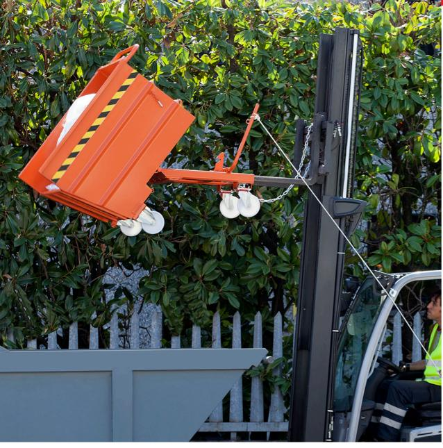
Heavy duty forklift tipping skips for the waste materials collecting, handling and unloading with 4 wheels, reinforcements and capacity up to 2000 kg. The operator activates the emptying mechanism within the forklift with no need to get out.
