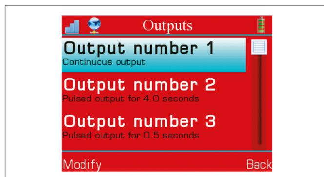
The **output type selection screen** contains 2 types of output:
