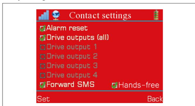
The contact settings are for assigning special remote control privileges to some contacts or forwarding messages the **GSM-00** receives to the corresponding number:
