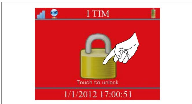
To unlock the dialler, tap the padlock in the centre of the screen and enter the administrator password (default setting "12345") using the touch keypad. Then tap confirm in the bottom right corner.
