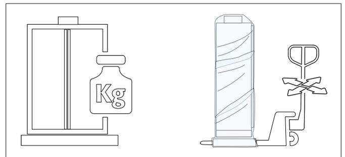
Use a pallet truck to move the product, which must be placed vertically and be secured and protected against slipping up to its final installation site.
