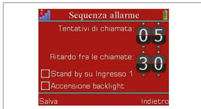
If “Standby on input 1” is ticked, input 1 works as a total dialler block, so it will not react to any alarm while this input is in alarm state. In these conditions, “Standby” appears on the main display to signal the dialler is not active. In the status SMS (“status” command), the text “StBy enabled” was added to the “System:” row if the function was enabled from the menu. The system status (standby or otherwise) is therefore visible on the “Inputs” row.
