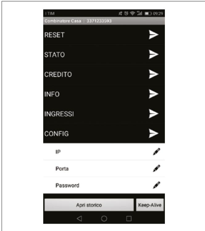
The “Keep-Alive” button at the bottom right of the screen allows you to set up a monitoring system based on “STATUS” messages. The dropdown menu is for selecting the operating mode.
