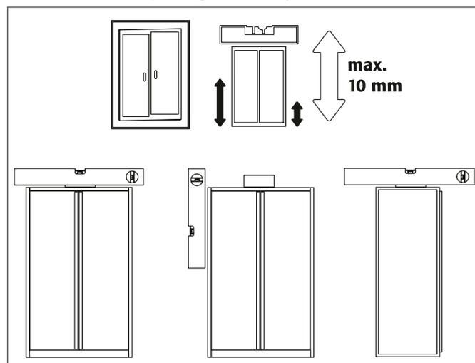
If necessary, level the product by adjusting the support feet.
