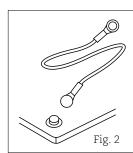
For optimum electrical performance, the mat should be cleaned regularly with a mild detergent of anti-static cleaner. **DO NOT USE CLEANERS WITH SILICONE**. This will build up a silicone coating on the mat which will cause the surface to become an insulator.
