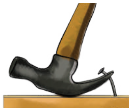
Back end of a hammer to remove a nail
